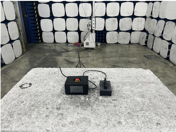
Radiated Emission Test Set-up for 30M-1GHz
