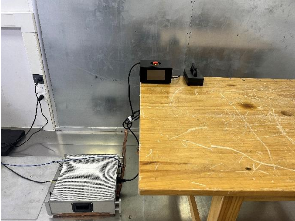
Radiated Emission Test Set-up for 30M-1GHz
