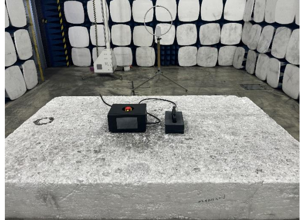
Radiated Emission Test Set-up for Below 30MHz
