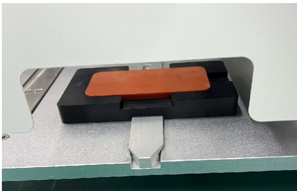
Pic 6.2-2 推入载具 push the carrier
