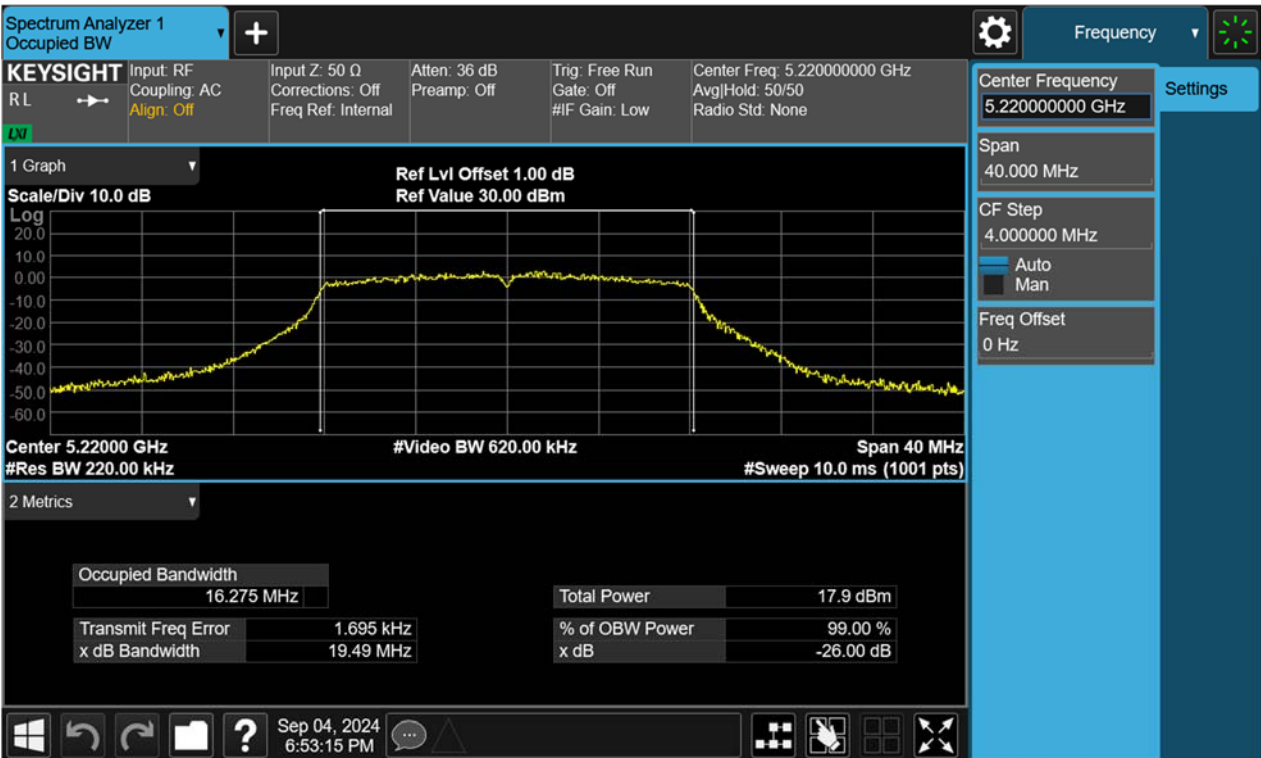
Figure 2: 802.11a, 5220MHz Test Plot of -26dB Bandwidth and 99% Bandwidth
