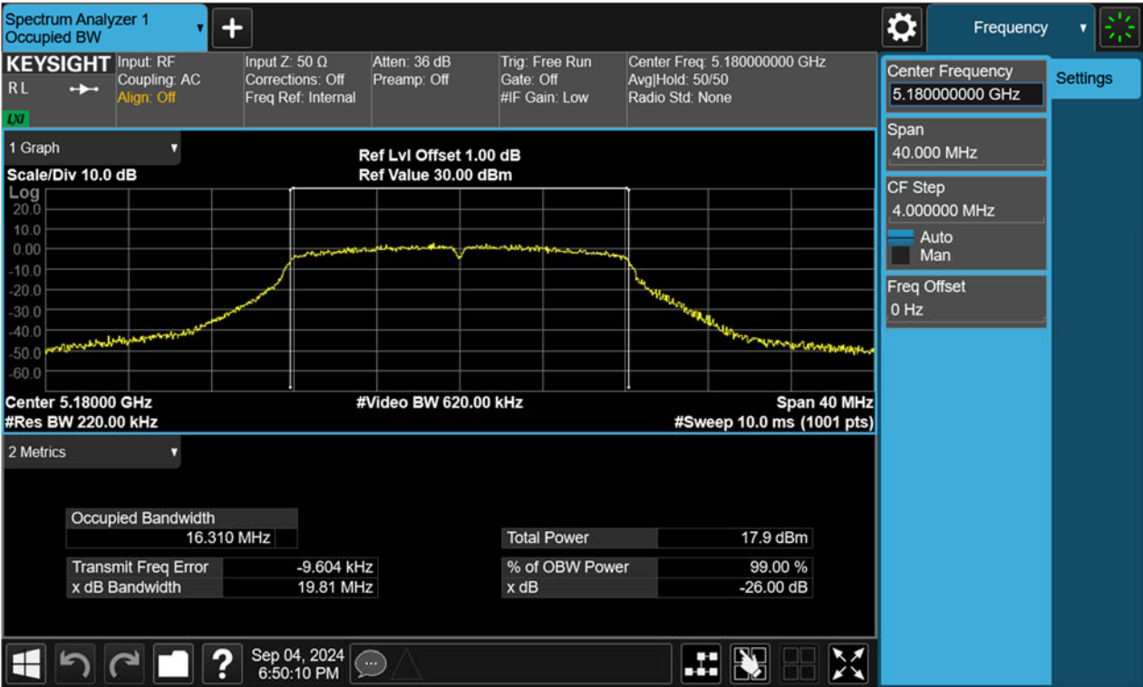
Figure 2: 802.11a, 5220MHz Test Plot of -26dB Bandwidth and 99% Bandwidth
