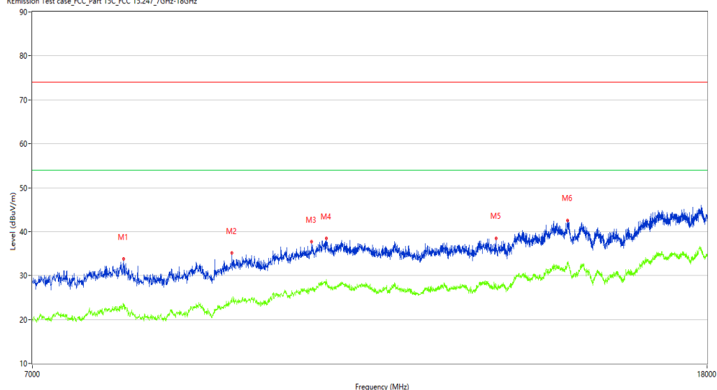
REmission Test case_FCC_Part 15C_FCC 15.247_7GHz-18GHz
