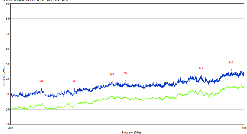
REmission Test case_FCC_Part 15C_FCC 15.247_7GHz-18GHz
