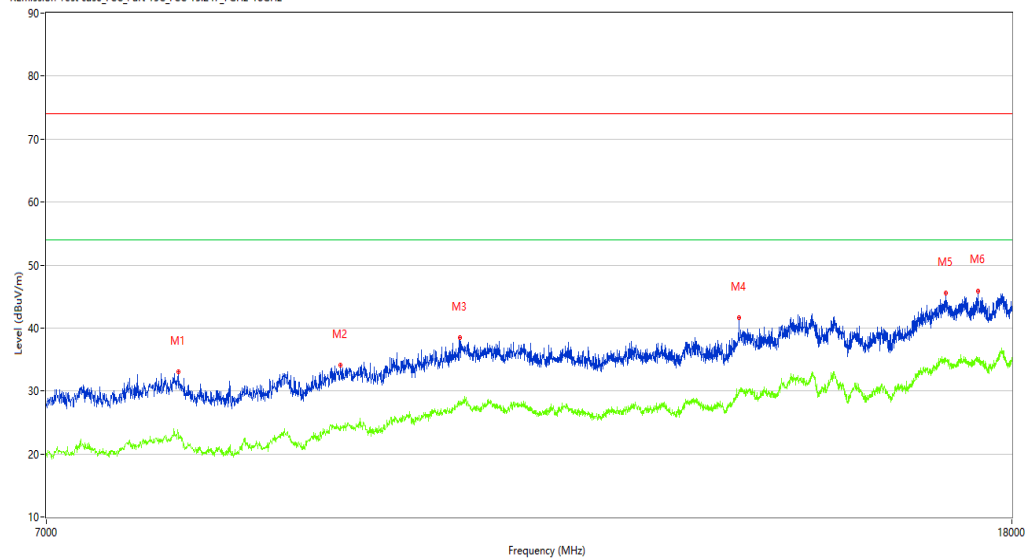
REmission Test case_FCC_Part 15C_FCC 15.247_7GHz-18GHz
