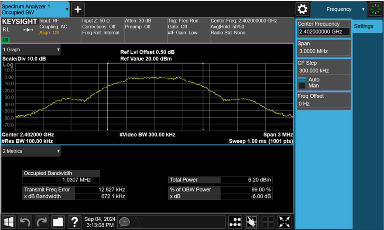
Figure 4: 6dB Bandwidth, 2402MHz
