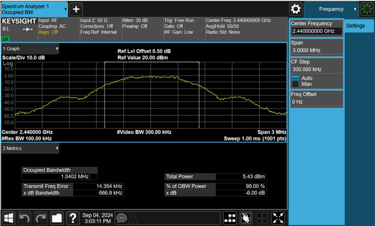
Figure 6: 6dB Bandwidth, 2480MHz
