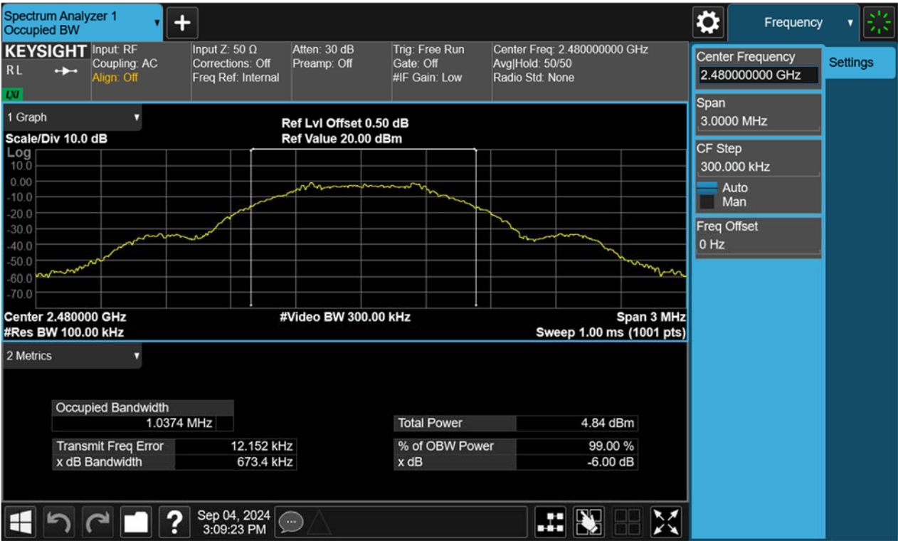
Figure 6: 6dB Bandwidth, 2480MHz
