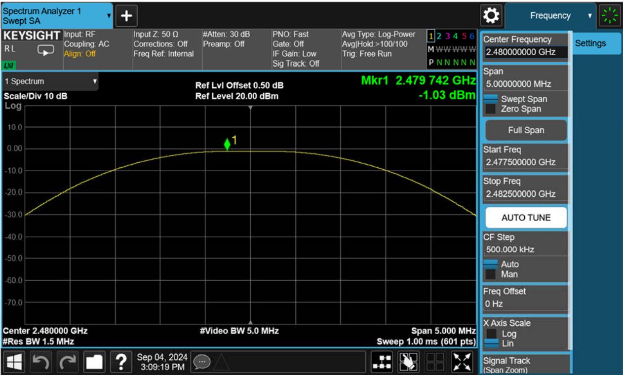
Figure 3: Peak Output Power, 2480MHz
