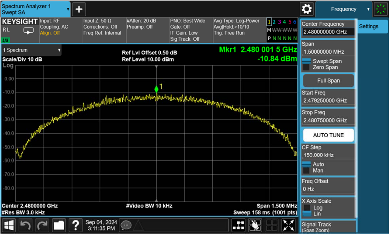
Figure 9: Power Spectral Density, 2480MHz
