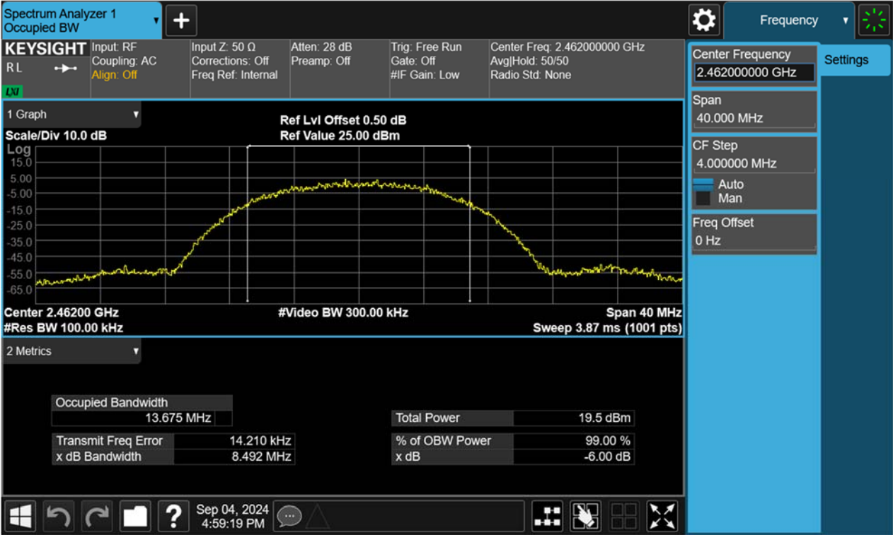
Figure 4: 6dB Bandwidth, 802.11g, 2412MHz
