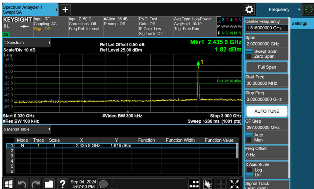
Conducted spurious emissions 30MHz-25GHz
