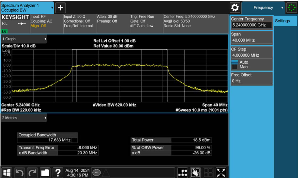
Figure 6: 802.11n(HT20), 5240MHz Test Plot of -26dB Bandwidth and 99% Bandwidth
