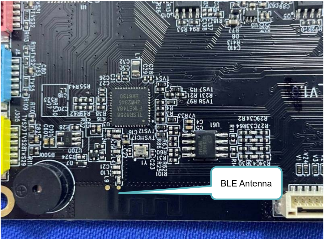
Bluetooth LE—Antenna Position
