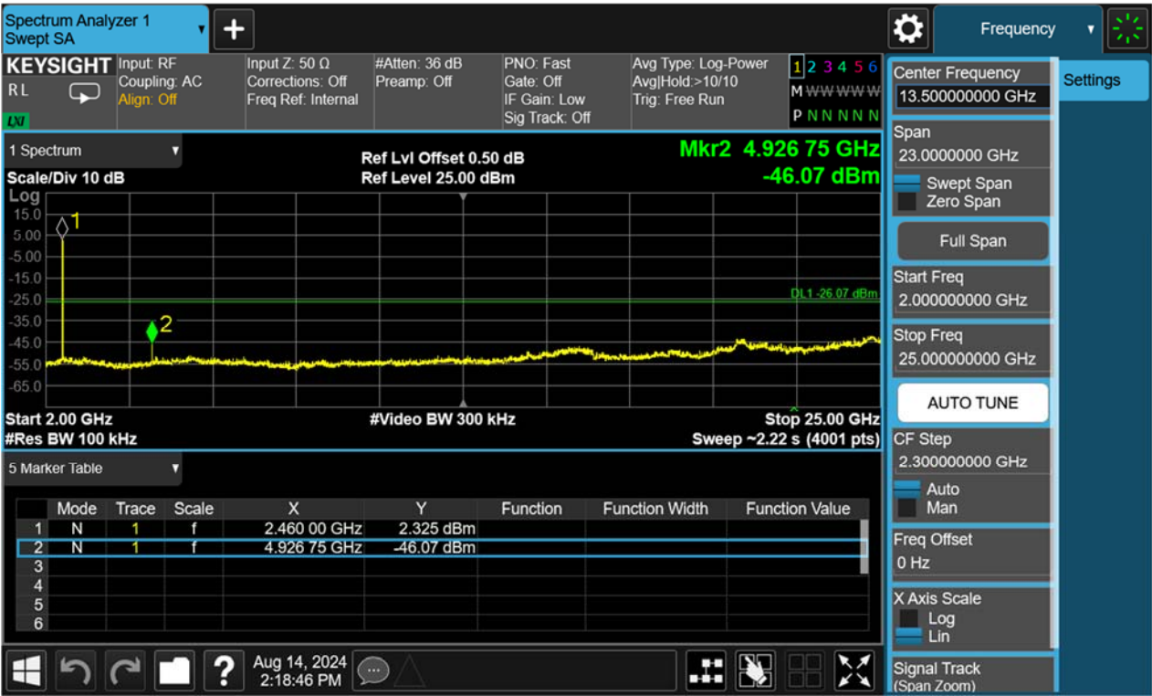
Figure 22: Conducted Spurious Emission & Authorized-band band-edge, 802.11g, 2412MHz Carrier Level
