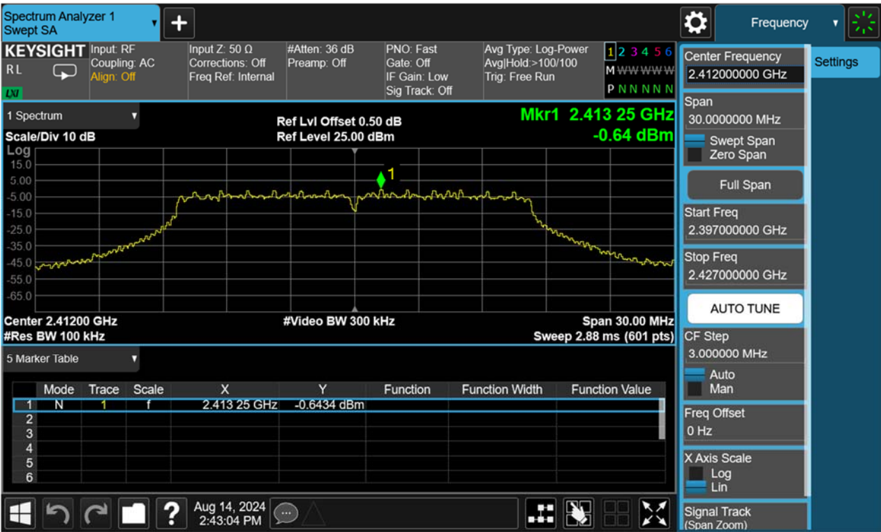
Figure 22: Conducted Spurious Emission & Authorized-band band-edge, 802.11g, 2412MHz Carrier Level
