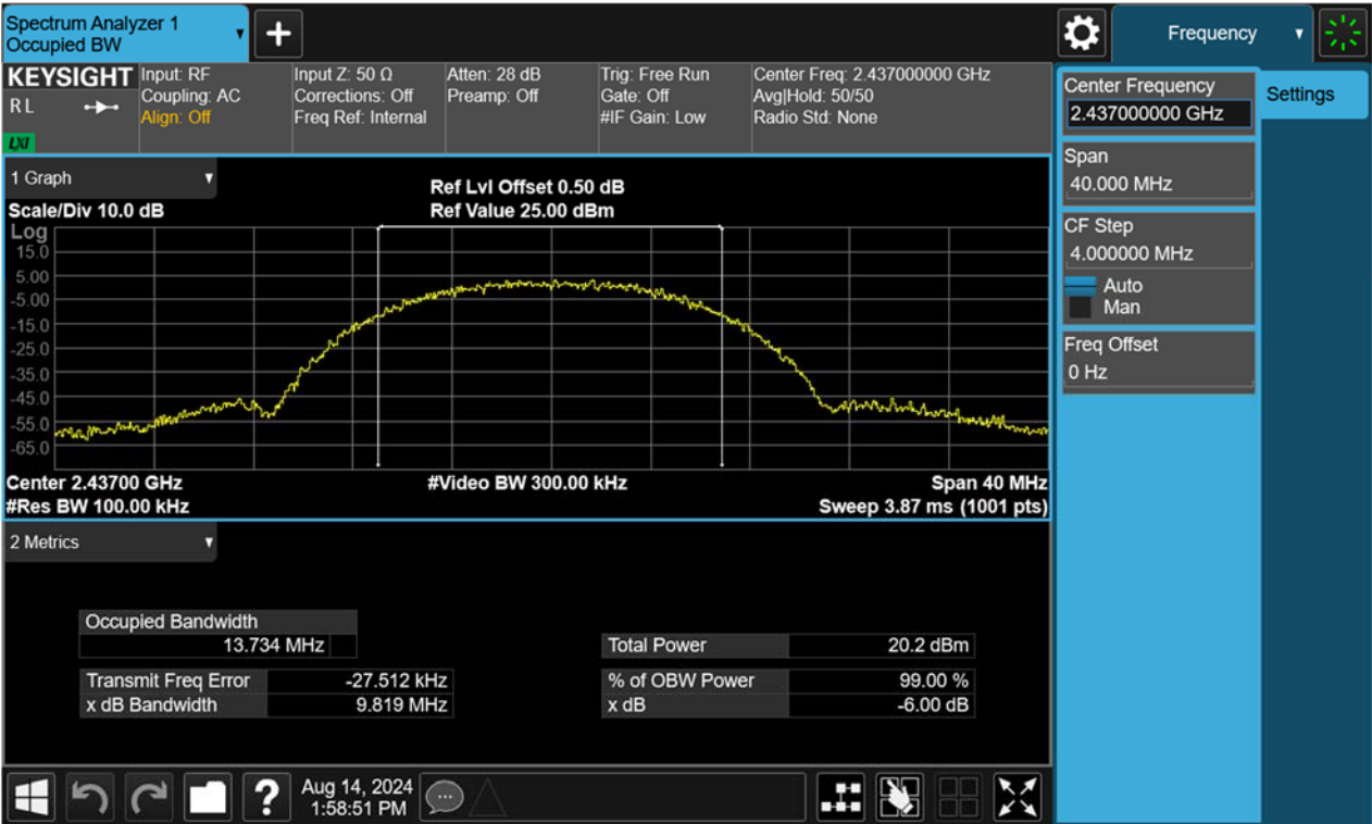
Figure 2: 6dB Bandwidth, 802.11b, 2437MHz
