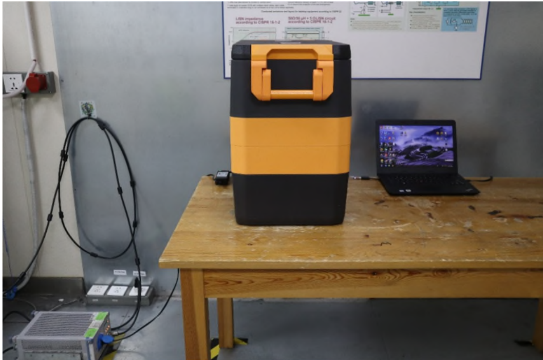
Photograph 3: Set-up for Conducted Emission
