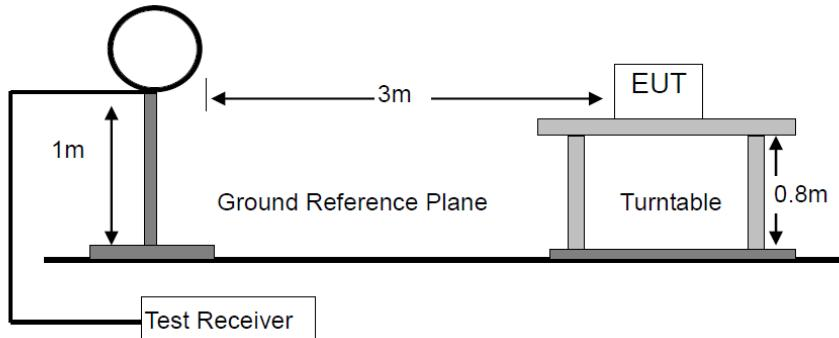
For Radiated Emission 30-1000MHz
