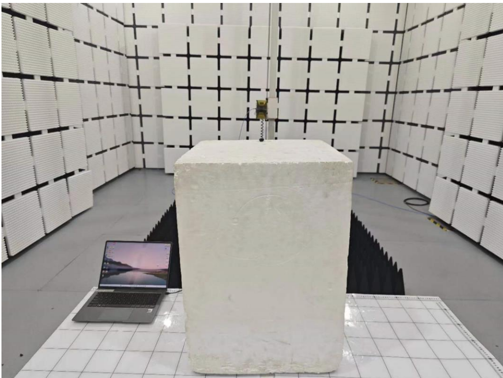
Set-up for Radiated Spurious Emission, Above 1GHz
