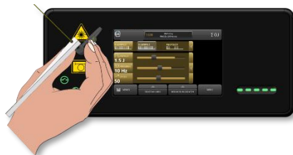
Fig. 44: Insert the fiber into the beam aperture and carefully screw it in tightly
