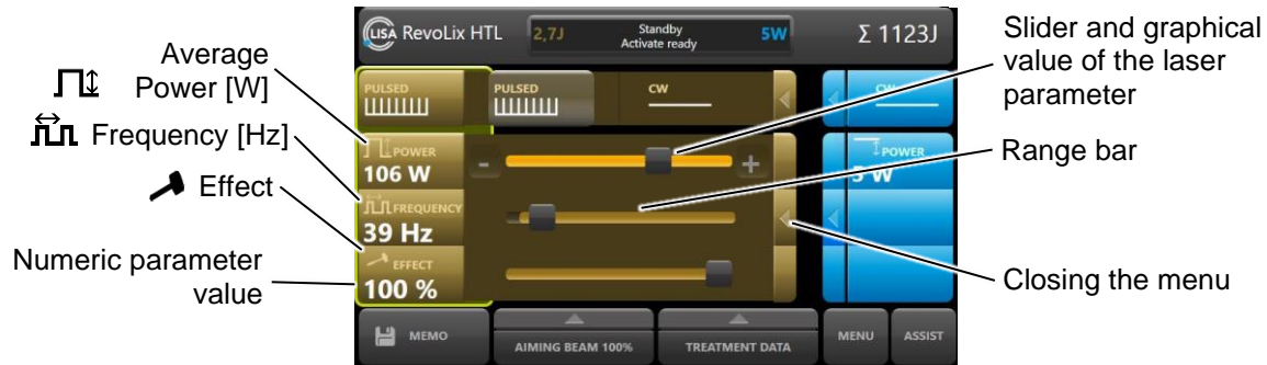
Fig. 30: Setting of the laser parameters; here in the PULSED operating mode
