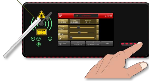
Fig. 50: Active laser warning light ribbon in LASER READY state
