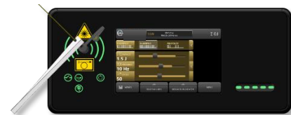
Fig. 43: Beam aperture opens automatically
