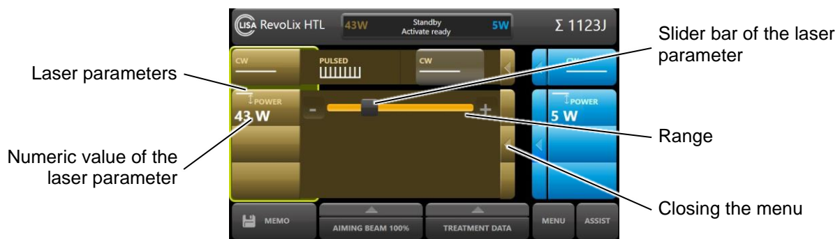
Fig. 29: Setting of the laser parameters; here in CW mode
