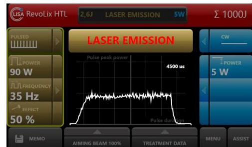
Fig. 32: Pulse shape of a long laser pulse with a low pulse peak power
