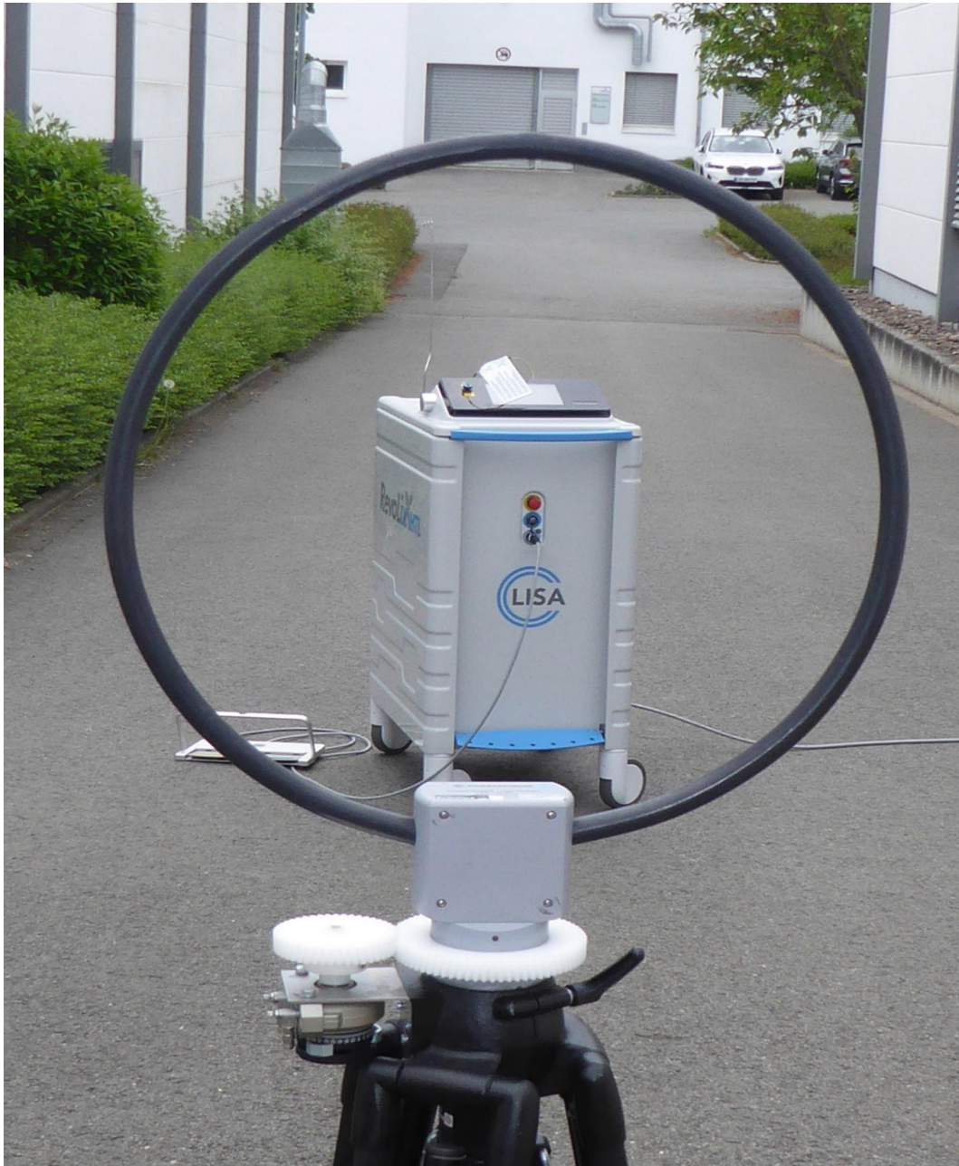
220394_02 : Test setup final measurement 9 kHz – 30 MHz
