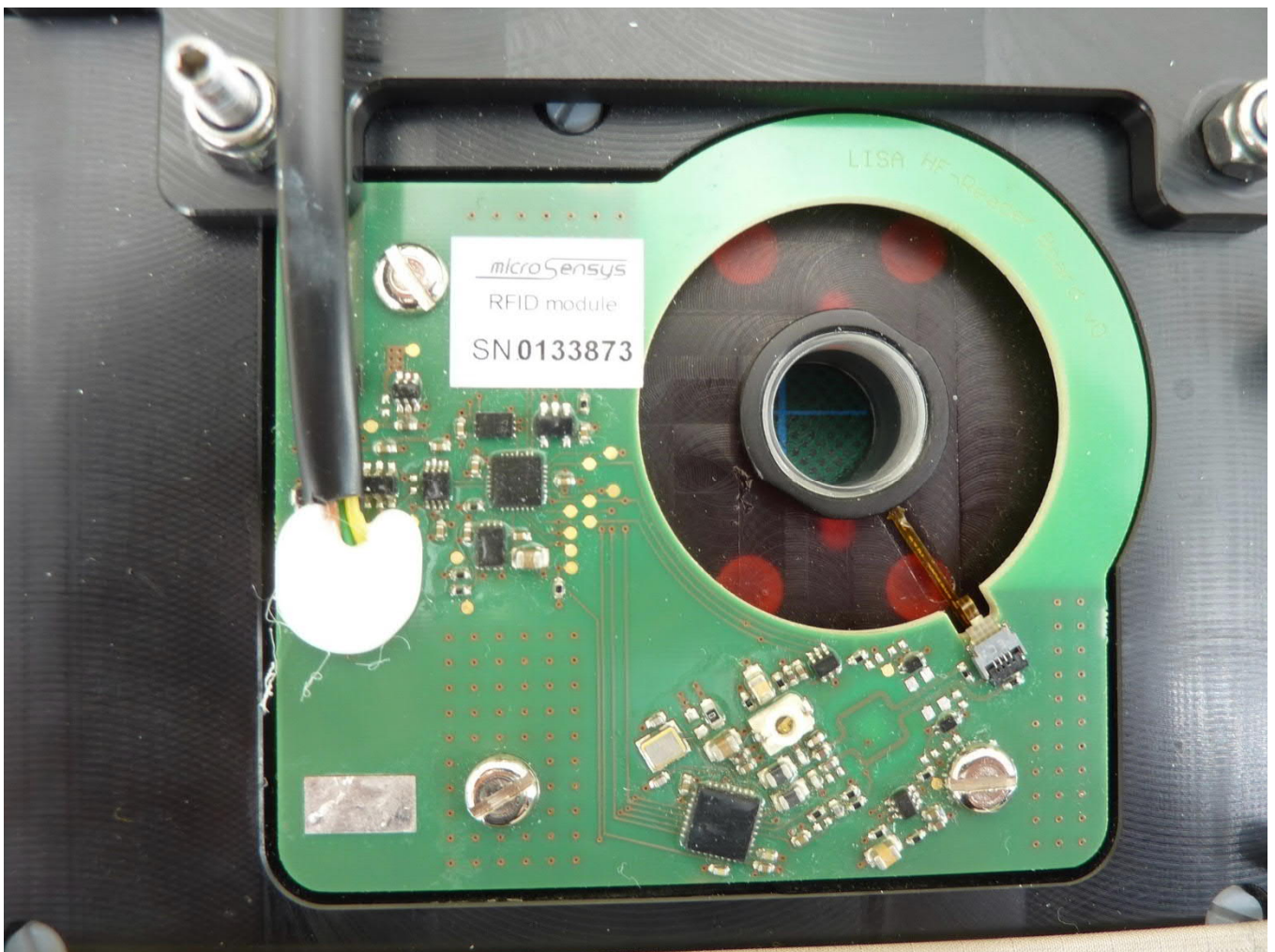
220394_EUT22: RFID reader rear view
