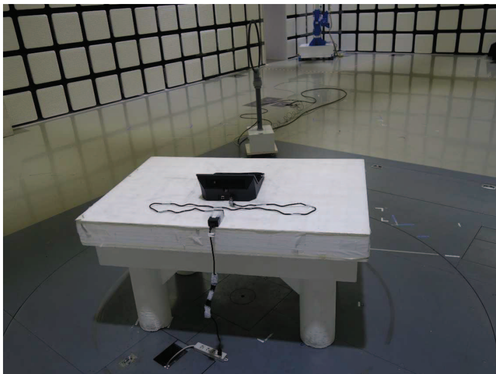
Photograph 9: Set-up for Radiated Emission of Transmitter Below 30MHz, Rear View
