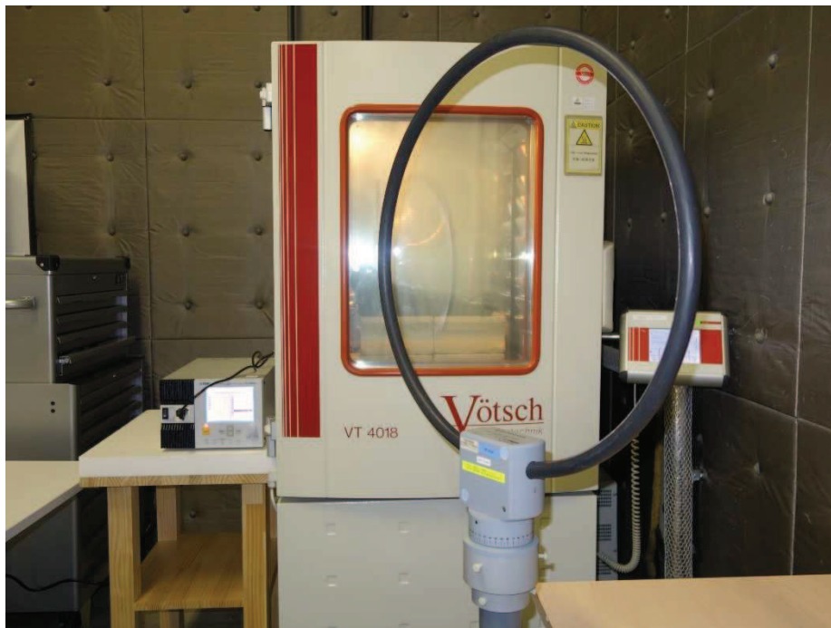
Photograph 4: Set-up for Frequency Stability, General View
