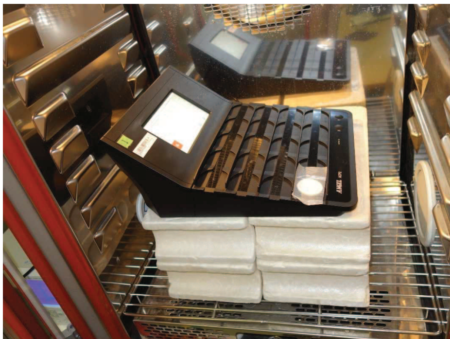
Photograph 5: Set-up for Frequency Stability, inside Temperature Chamber
