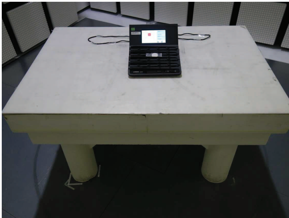
Photograph 10: Set-up for Radiated Emission of Transmitter, Front View
