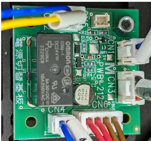
AC ~ battery Controller
