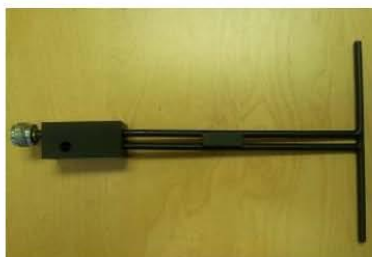
Figure 1 – MVG COMOSAR Validation Dipole
