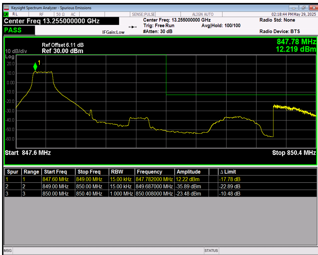
Band5 64QAM BW=1.4MHz Channel=20643 RB Size=1 Position=#Max
