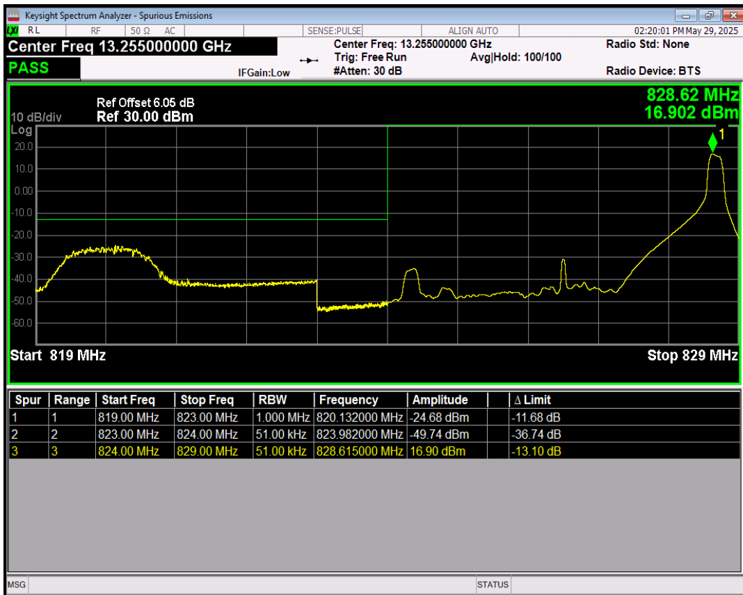
Band5 64QAM BW=5MHz Channel=20425 RB Size=25 Position=#0
