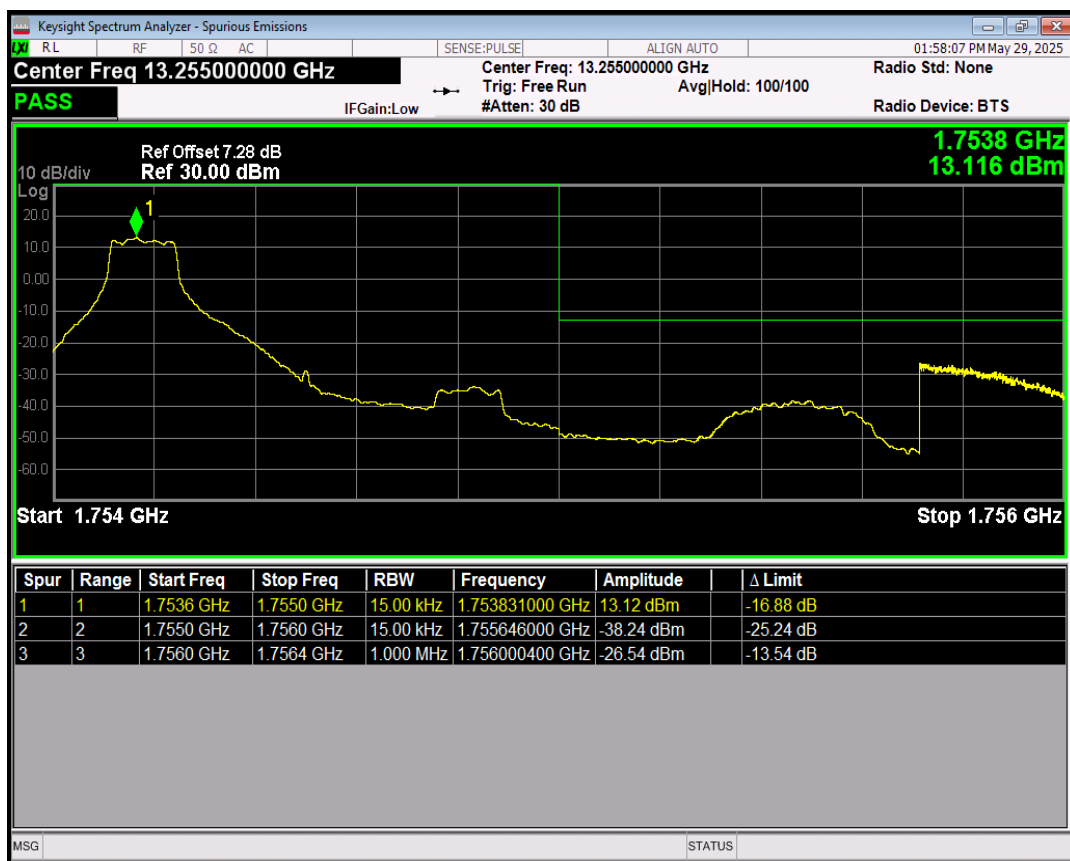
Band4 16QAM BW=1.4MHz Channel=20393 RB Size=1 Position=#Max
