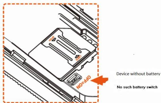
② Disconnect the external power supply and turn the backup battery switch to the OFF position, and the terminal will shut down. After shutting down, the power indicator will go out and the internal battery will stop charging.
