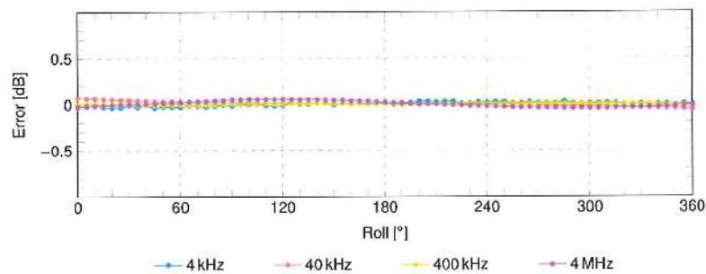
SPEAG axial deviation from the ideal response tolerance for H-field:  $\pm 0.6$  dB
