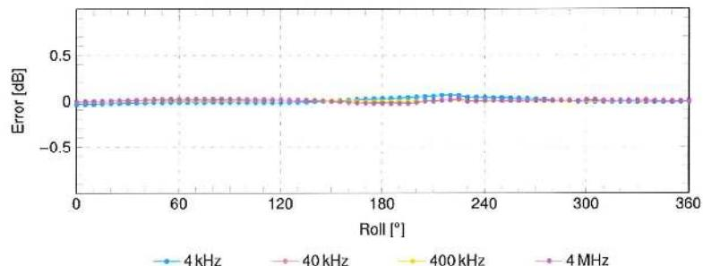
SPEAG axial deviation from the ideal response tolerance for E-field:  $\pm 0.8\text{dB}$
