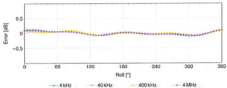
**E-Field Receiving Pattern ( $\phi$ ),  $\theta = 90^\circ$**
