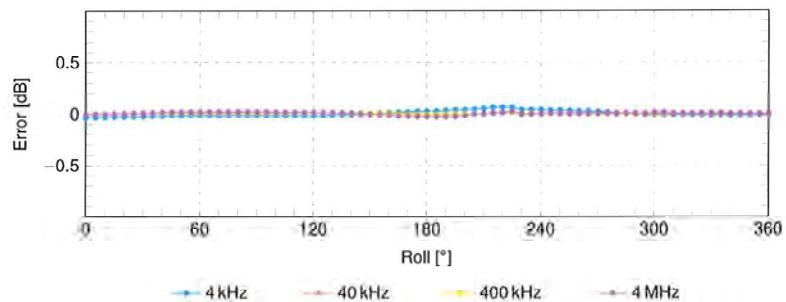
SPEAG axial deviation from the ideal response tolerance for E-field:  $\pm 0.8$  dB
