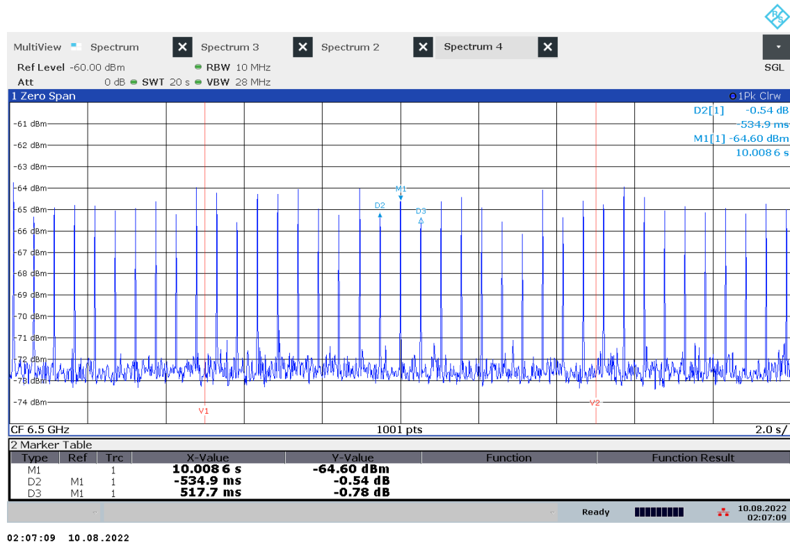
Plot 15: Emission of EUT without associated receiver (for comparison), normal mode
