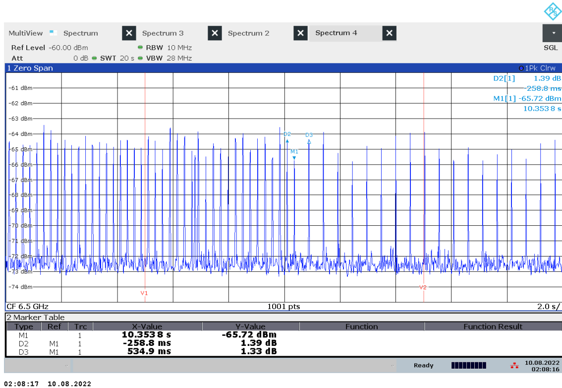
Plot 14: Emissions of the EUT, only at the beginning with associated receiver (normal mode)
