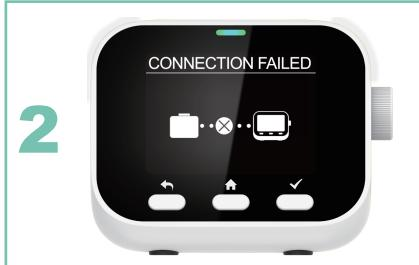
2. If it shows that the connection failed, move the device close to the base station and **restart** the monitor device to reconnect.
