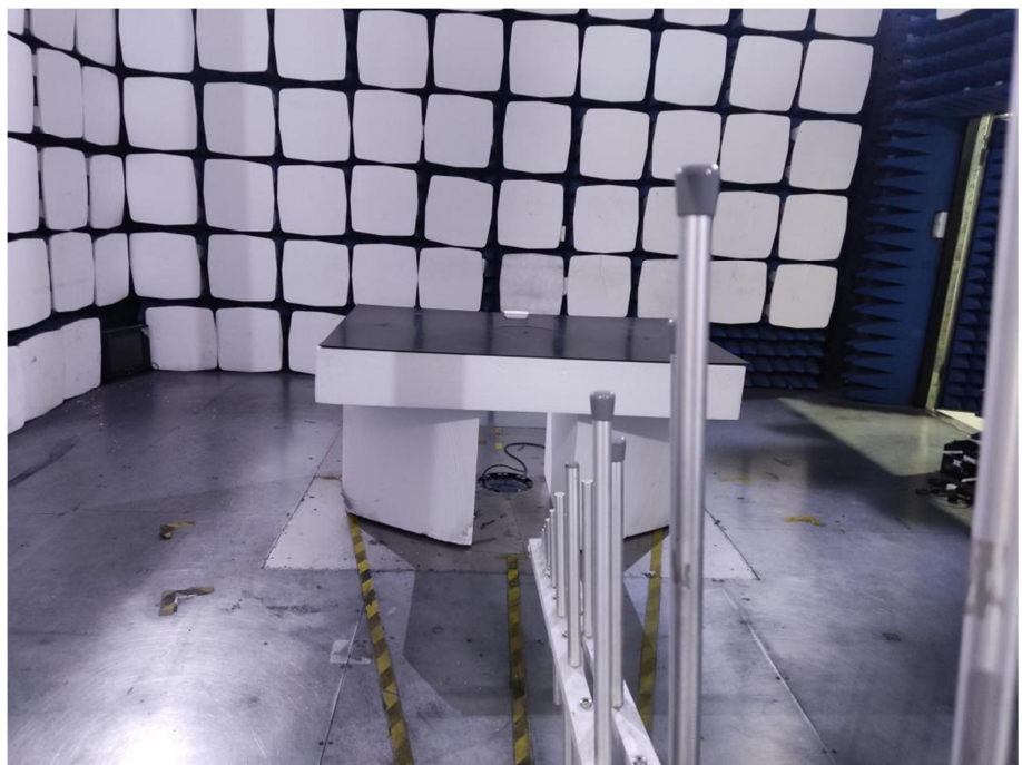
Radiation Emission Test Setup (30MHz to 1GHz)
