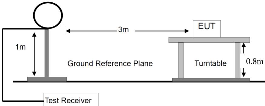
For Radiated Emission 30-1000MHz
