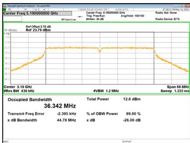
(802.11ac40) plot on channel 46
