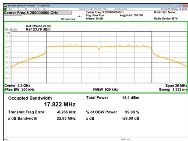
(802.11ac20) plot on channel 48
