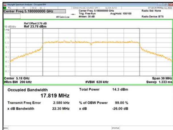
(802.11ac20) plot on channel 40
