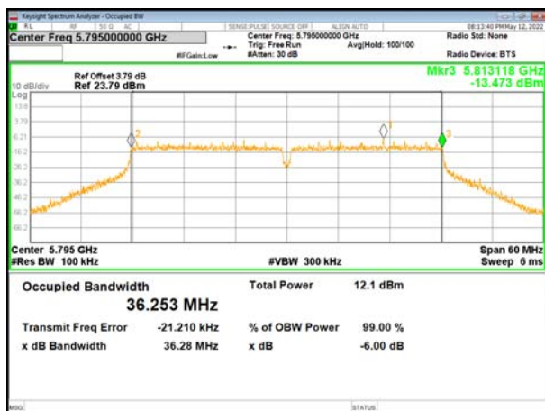
(802.11 ac40) plot on channel 159
