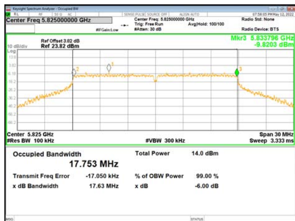
(802.11ac20) plot on channel 165
