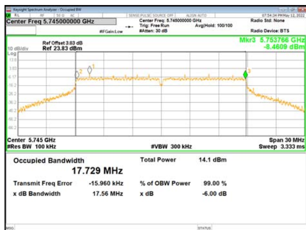
(802.11ac20) plot on channel 157
