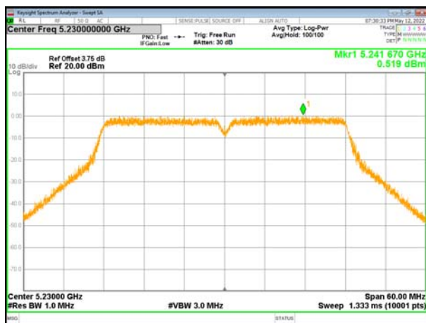
(802.11ac40) PSD plot on channel 46
