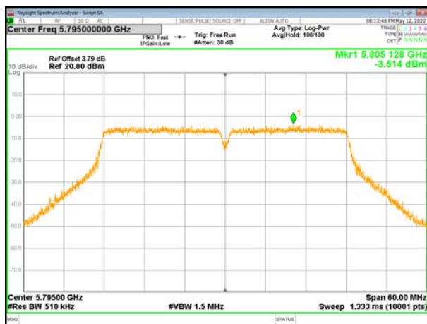
(802.11ac40) PSD plot on channel 159
