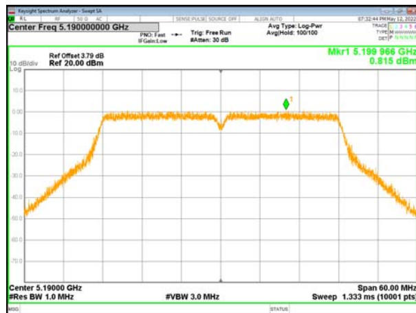
(802.11n40) PSD plot on channel 46
