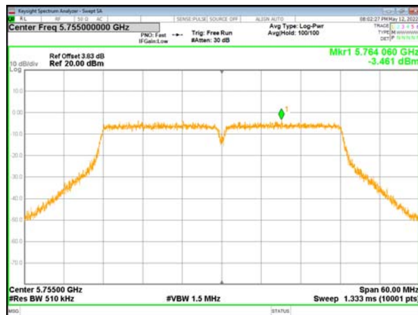
(802.11n40) PSD plot on channel 159
