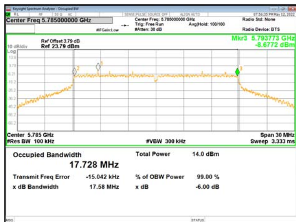
(802.11ac20) plot on channel 165
