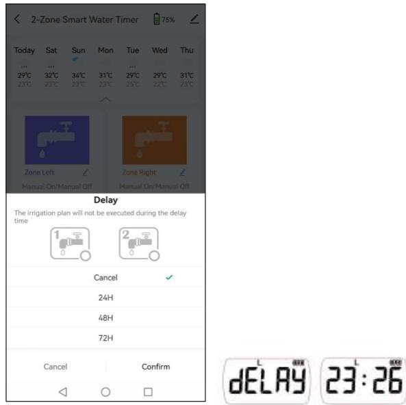
Note: When the left/right valve is in the delay state, the timer device will display the "DELAY" icon on the screen, and then display the remaining time at an interval of 3 seconds.
