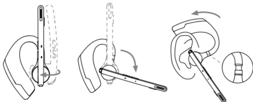
② Rotate the microphone boom to ensure the microphone
