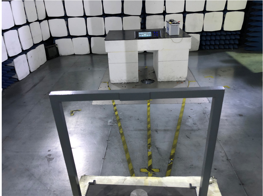
Radiation Emission Test Setup (Below 30MHz)
