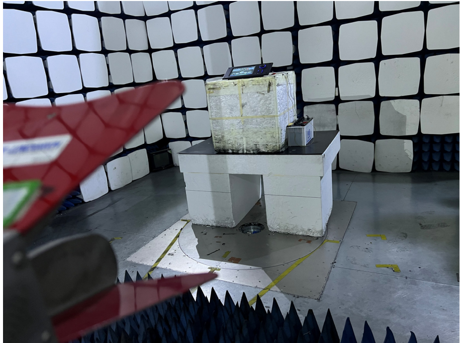
Radiation Emission Test Setup (1GHz to 18GHz)
