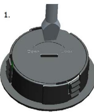
Unscrew the remote control battery cover as shown in the figure
