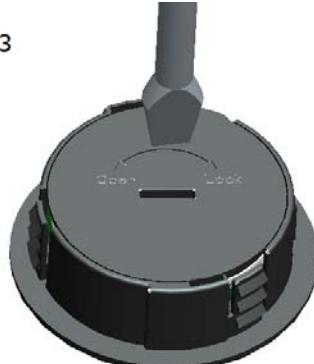
Tighten the battery cover clockwise as shown
