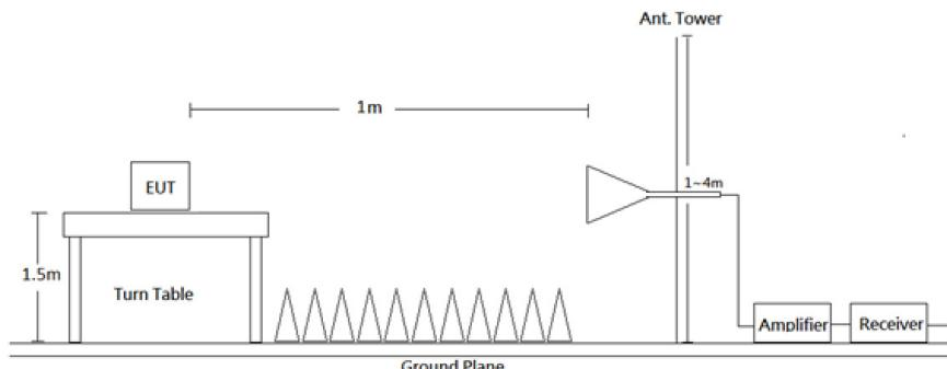
Radiated emission tests were performed in the 3 meters chamber test site, using the setup accordance with the ANSI C63.10-2013. The specification used was the FCC Part 15.209, FCC 15.247 Limits.
