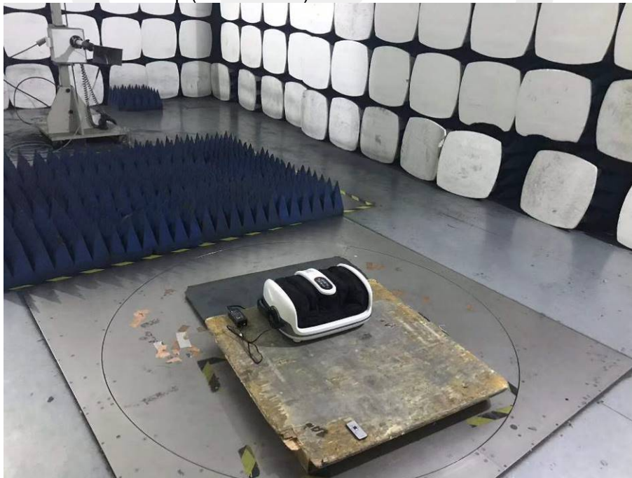
Spurious Emission Test Setup (Above 1GHz)
