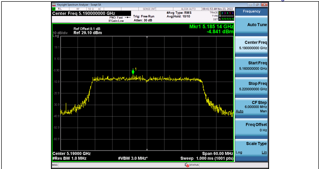
Power Spectral Density_5_2GWiFi_802_11ax(HE40)_5230_40M
