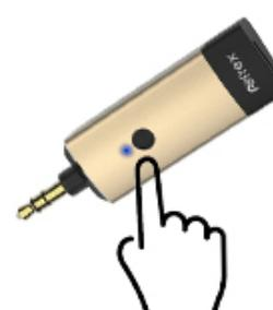
● Long press the button for 4 seconds until you see the LED light is flashing in blue rapidly ( blinks 5 times every second ), the Bluetooth transmitter will be automatically searching and pairing with your Bluetooth devices.
