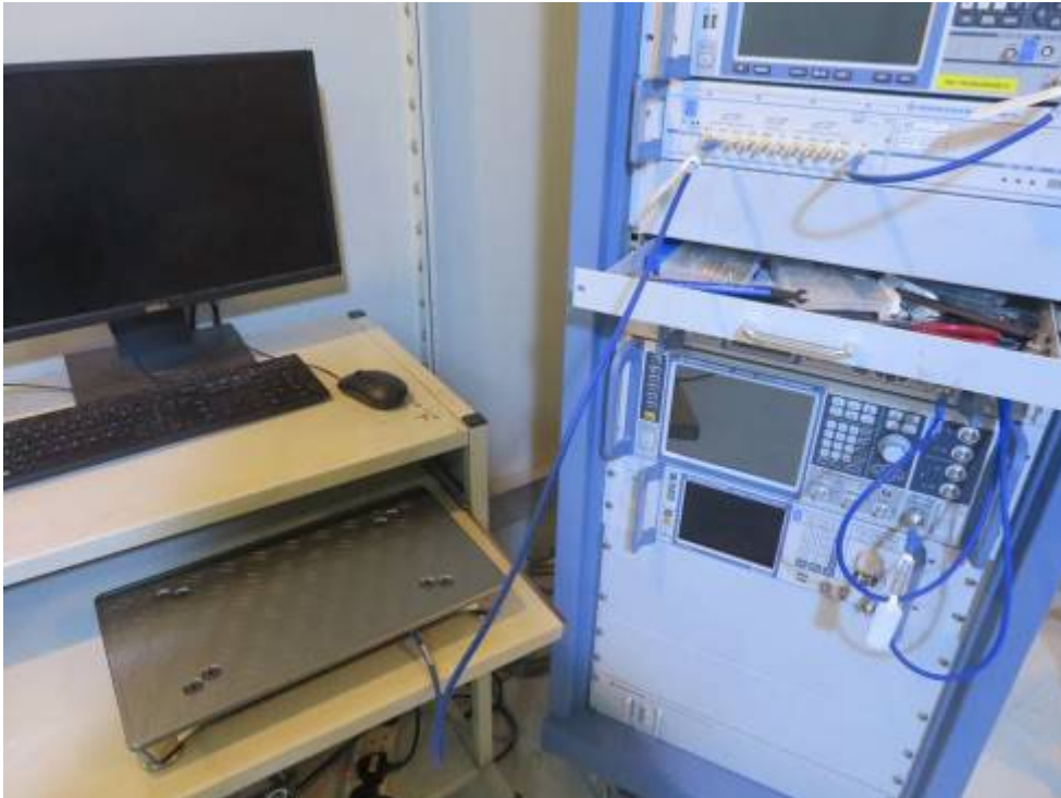
Conducted RF Output Power Test Setup
