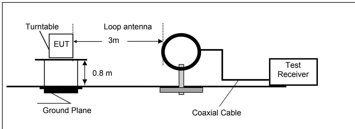
(B) Radiated Emission Test-Up Frequency 30MHz~1GHz
