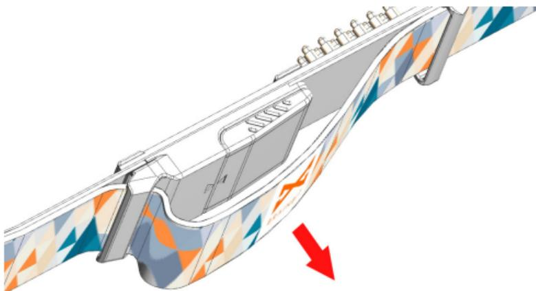
2. Holding the battery by the sides, release the battery.
