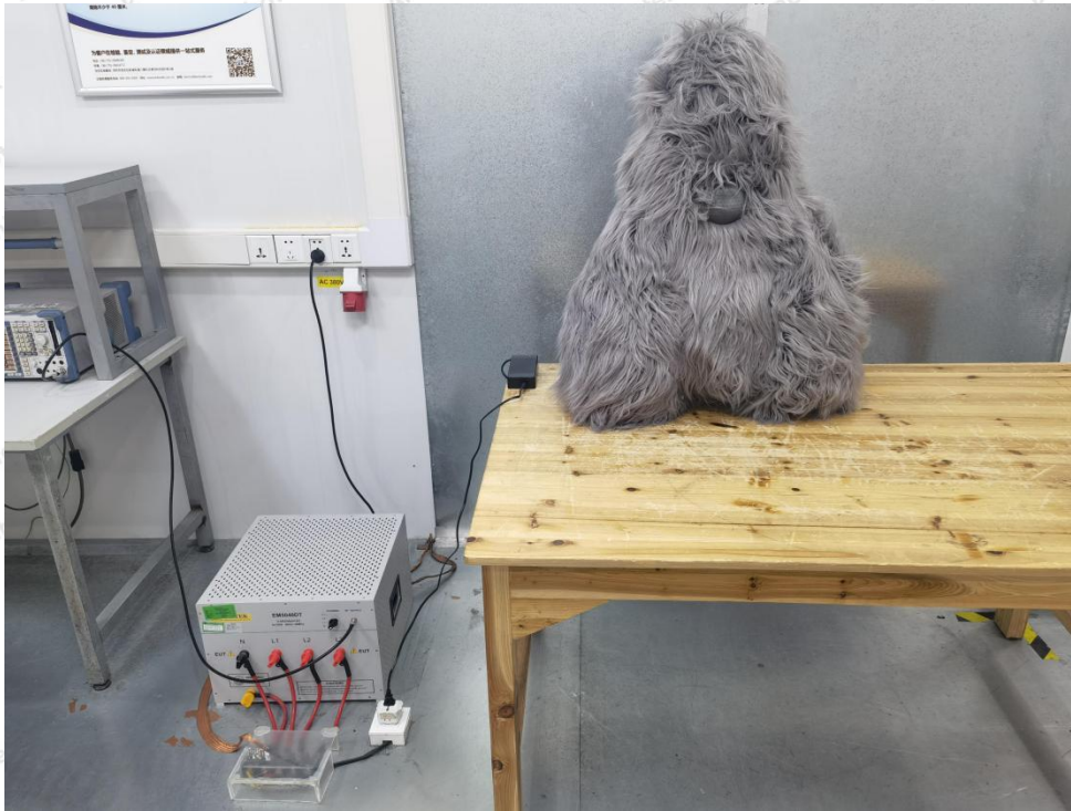
Photo of Conducted Emission Measurement
