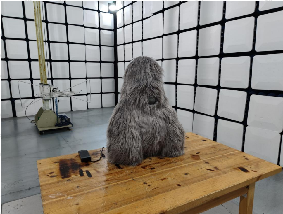
Photo of Radiation Emission Test
