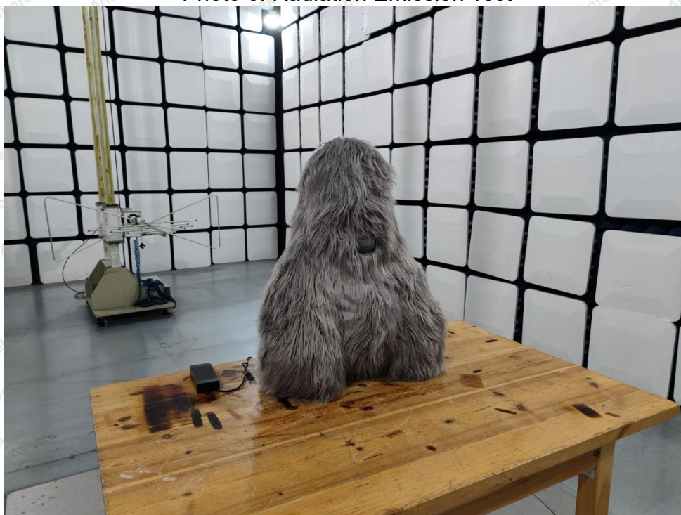
Photo of Radiation Emission Test
