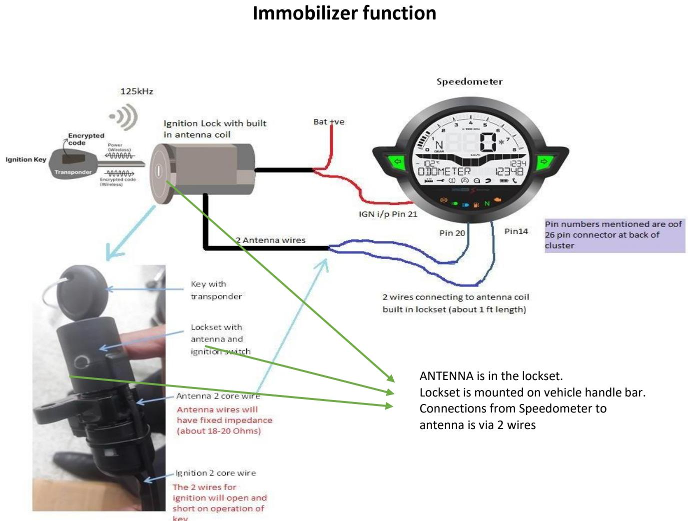
For enhanced safety, the vehicle start is not safeguarded only by mechanical key but also by Immobilizer function. Here digital authentication of valid user is carried out before the vehicle engine can start.
