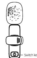
Step 3: The indicator red light of receiver keeps always on, then open the phone camera, live App or other Apps, and then to use the microphone to receive sound.
