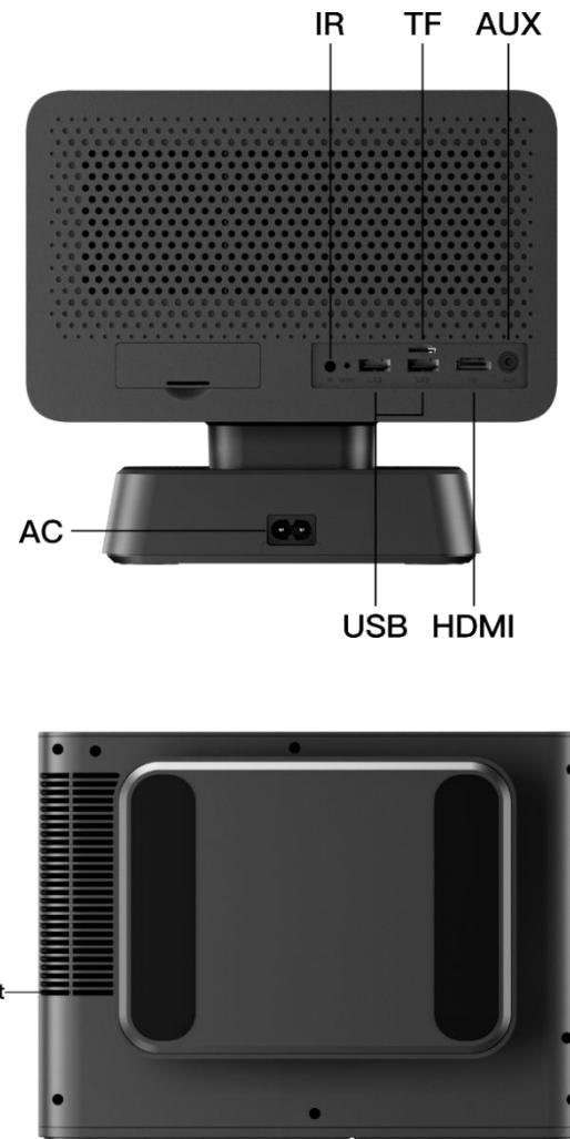
Do not block the air inlet and outlet.
