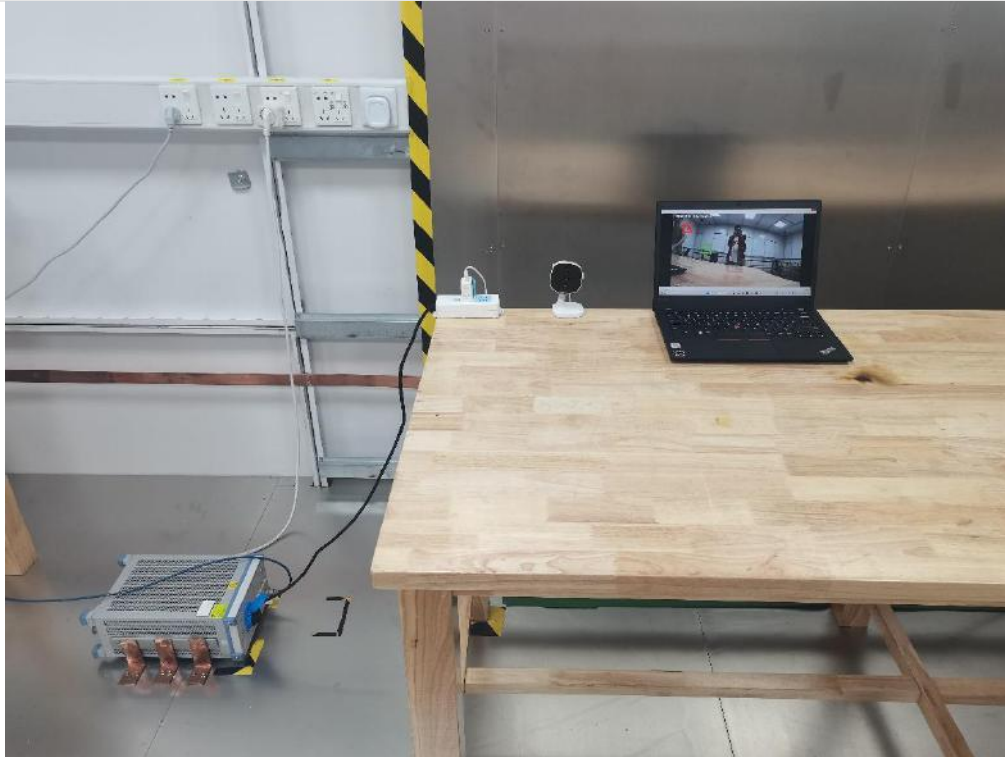
AC Power Line Conducted Emission
