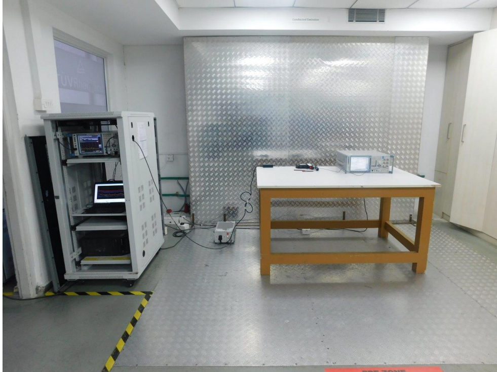
Conducted AC Powerlines Test setup
