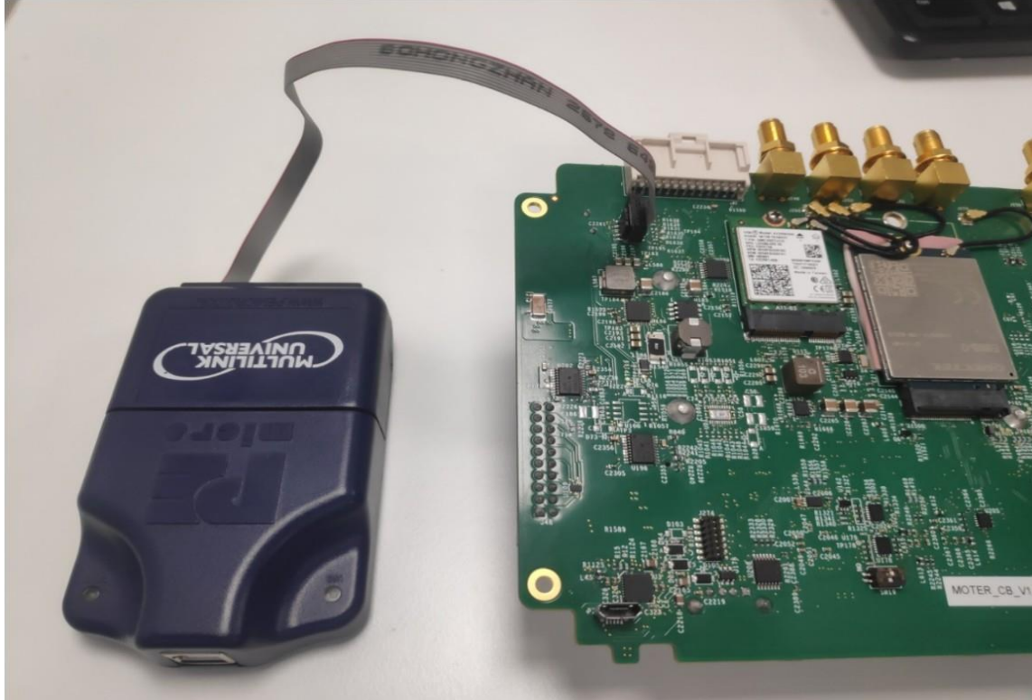
Figure 15 : JTAG and Board Cable Connection
