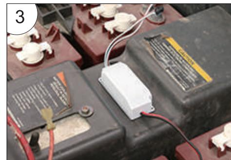
4. Connect the light wire to the Input Control box.
