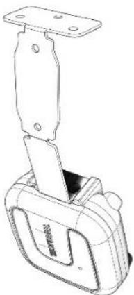
**Zone Anchor** : Ultra-Wide Band stationary devices used to slow down forklifts in designated zones. It is also used to track forklifts and pedestrian devices.
