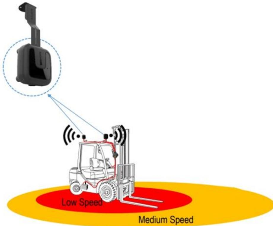
When there are people or forklifts in the low-medium-high risk areas around the forklift, the devices on the person and the forklift detect each other and the LEDs on the instrument panel give a warning. These distance settings are determined and sent according to the customer's request. It is possible to change them later.
