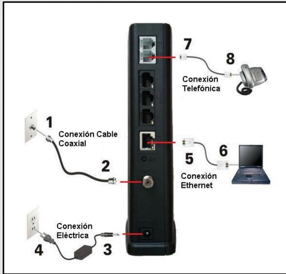
1. Connect the coaxial cable to the signal input
