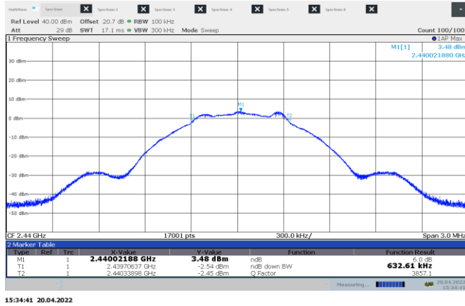
Figure 8.7-1: 6 dB bandwidth , sample plot
